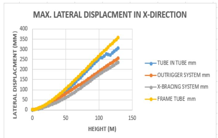
Fig. 7. Maximum lateral displacement in X-direction
