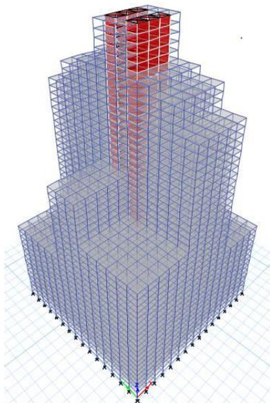
Fig. 6. 3D view of frame tube structure model
