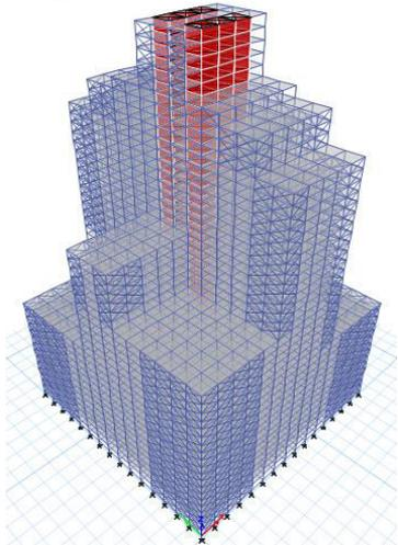
Fig. 5. 3D view of Braced frame structure model
