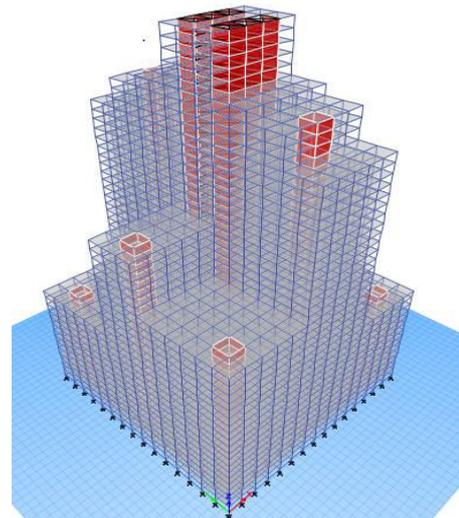
Fig. 3. 3D view of tube in tube structure model
