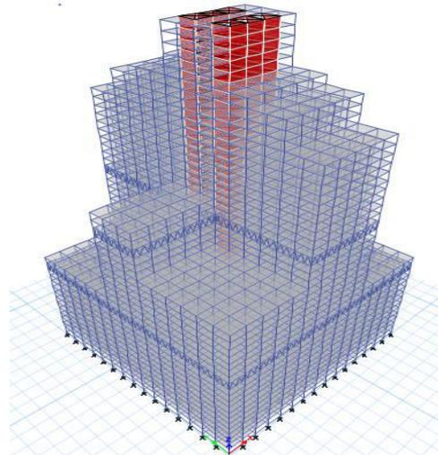
Fig. 4. 3D view of frame structure with outrigger system model
